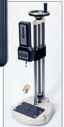
Optional Test Stand permits tension/compression analysis
